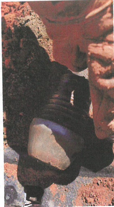
Evidence of LPH on the leading head of the core at 43 feet bgs.
