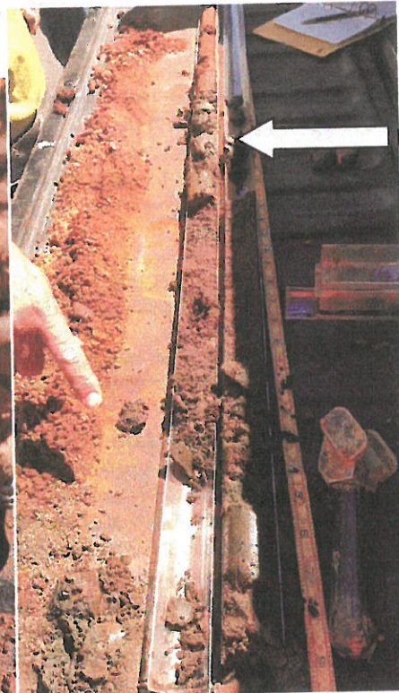
38 to 43 foot transition sleeve, arrow depicts the visual transition point. LPH saturated soils evident below the arrow.
