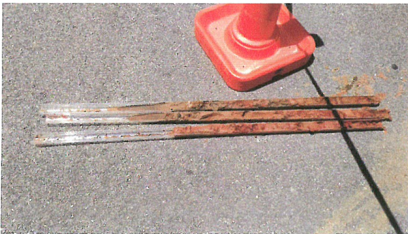
Soil cores collected below the water table in MW-52.
