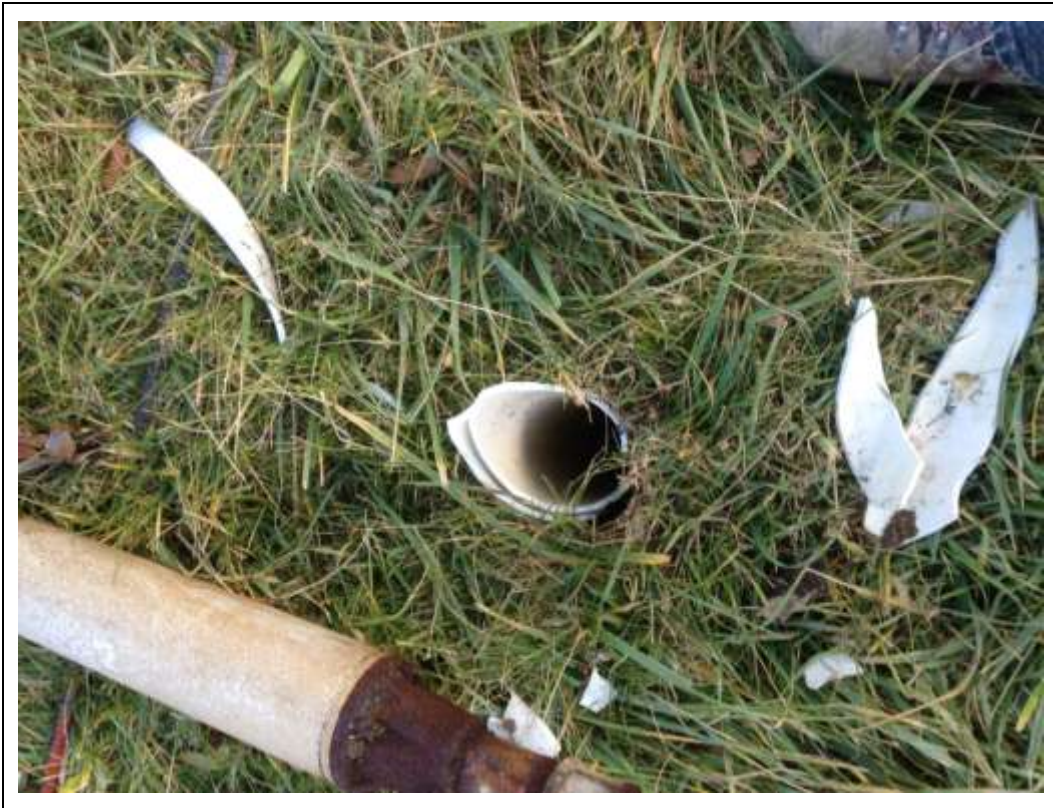
Photograph 7: Broken well casing on EMW-1
