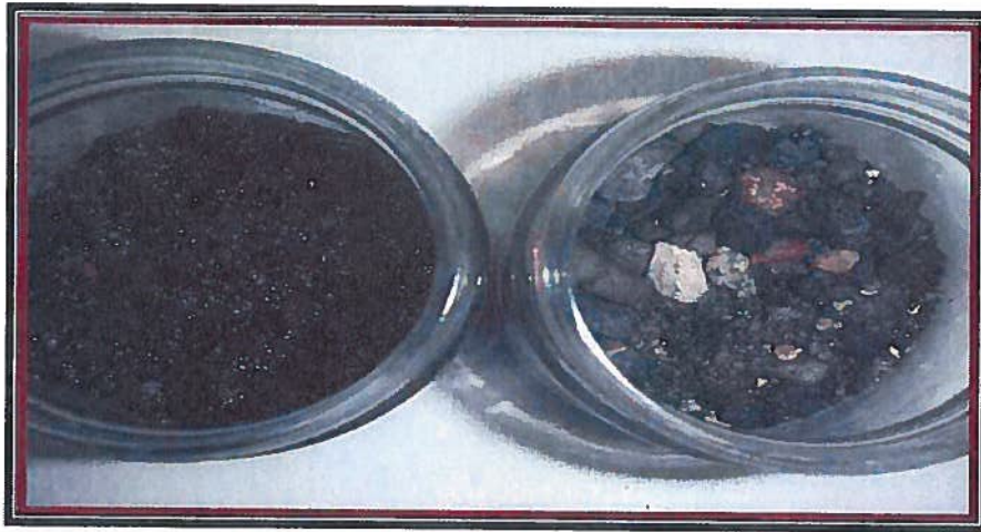
Photograph 2-1: Pre-post Ivey-sol ® Remediation of Refinery Soils
