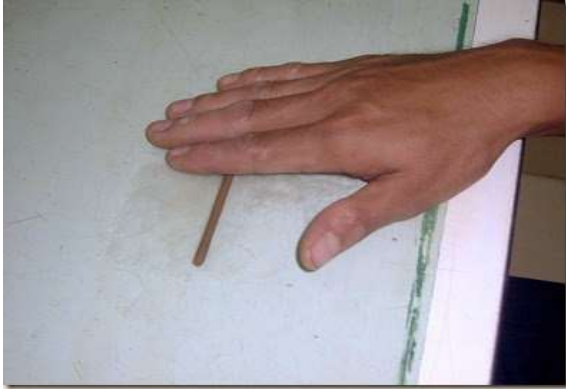
Rolling Clay to Determine Plasticity
