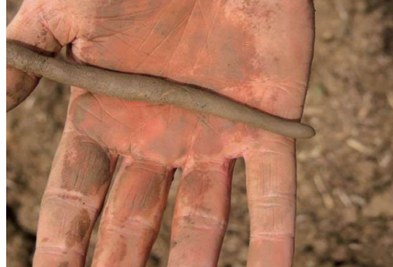
Rolling Clay in the Field to Estimate Plasticity
