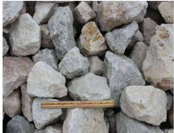
Loose Gabion Stone
